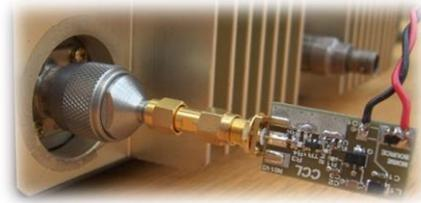
RXGen connected to 23cm antenna input
