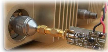
**RXGen connected to 23cm antenna input**
