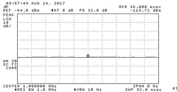
Here are two plots using HP 8596E with SAT1. Plot 1 noise marker indicates -171.8dBm, Plot 2 marker -113.7dBm/1MHz.
